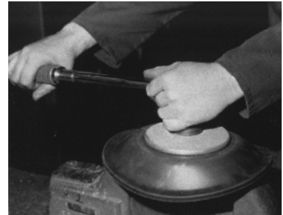
Figure 3: Torquing the diaphragm plate.
