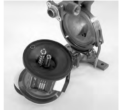
Disassembling the pilot valve.
