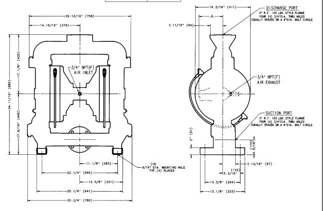
3" ASA-STYLE FLANGED SUCTION AND DISCHARGE • %"NPT(F) AIR INLET PORT • %" NPT(F) AIR EXHAUST PORT
