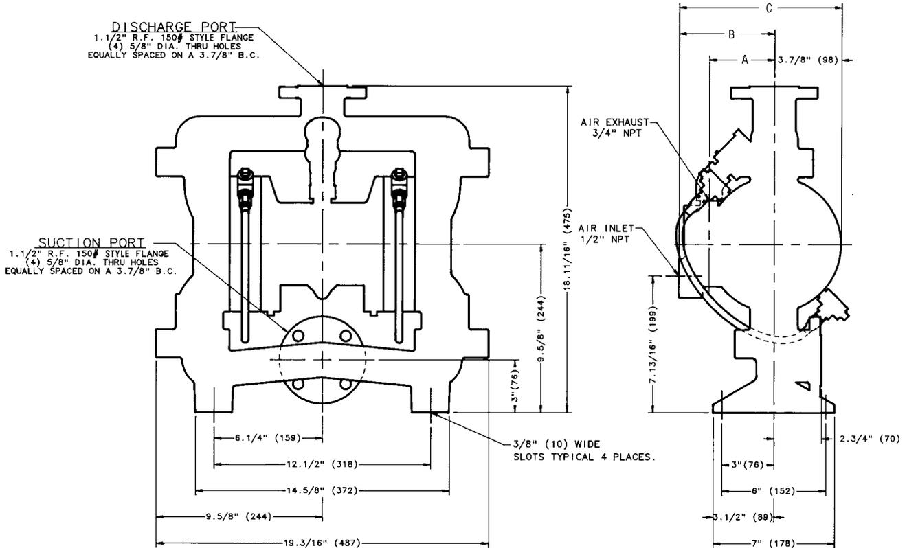
**1 1/2" ASA STYLE FLANGED SUCTION & DISCHARGE • 1/2" NPT(F) AIR INLET PORT • 3/4" NPT(M) AIR EXHAUST PORT**
