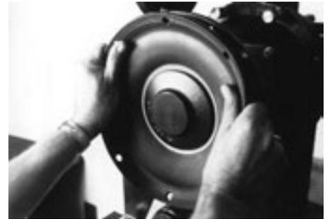
Figure 7: Align diaphragm holes with chamber holes
