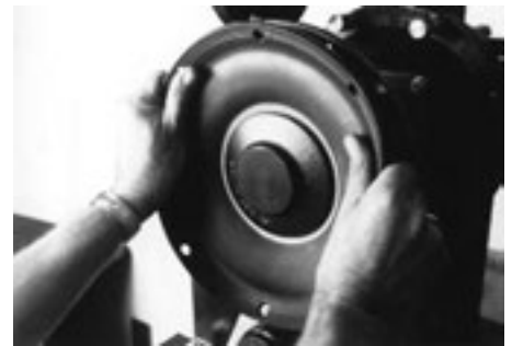
Figure 7: Align diaphragm holes with chamber holes
